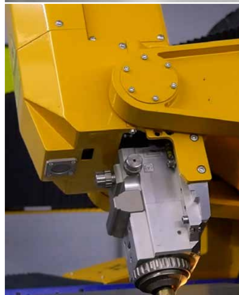
Laser bevel head allows 3D processing of sheets and pipes
