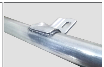
2mm aluminum pipe welding
