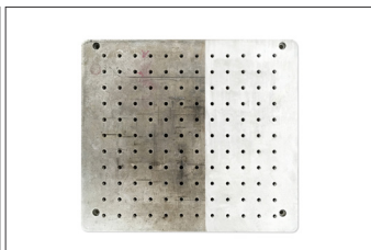
Aluminum alloy oxide layer cleaning
